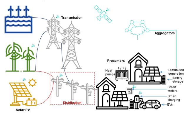
EXHIBIT 448: Electricity distribution networks integrate renewables and two-way flows and enable decarbonization of transport and heat
