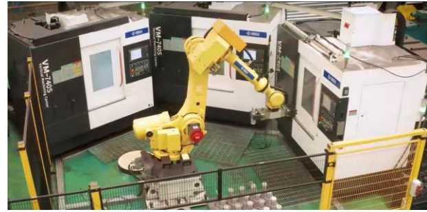
EXHIBIT 87: A single robot tending multiple machine tools (FANUC example)
