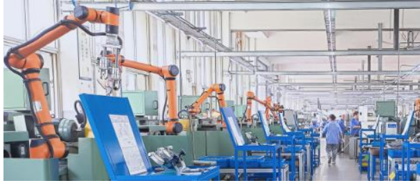
EXHIBIT 86: Cobot for machine tending (AUBO example)
